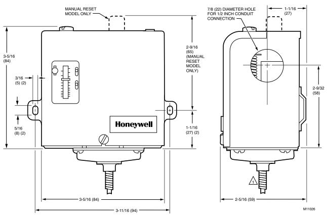
Fig. 1. L480 Temperature Controller dimensions in in. (mm).
