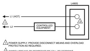
SWITCH BREAKS ON TEMPERATURE FALL TO SETPOINT. MUST BE MANUALLY RESET.
