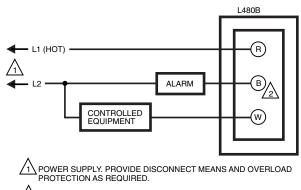
2 SWITCH MAKES R-B, BREAKS R-W ON TEMPERATURE M11039 FALL TO SETPOINT.
